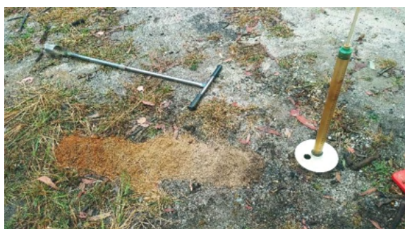
View of a permeameter insitu in LCA test area. The land application area has a slope of approximately 8% with fair solar and wind exposure, soil had reasonable permeability
